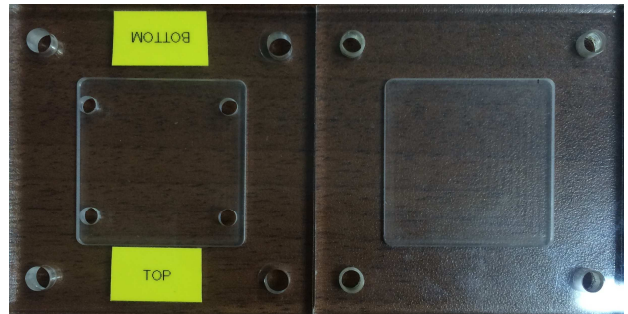
Fig. 5 The mask of device that PDMS and AAO bonding by using Acrylic plastic frame
